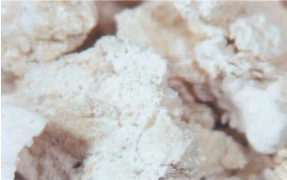
Fig. 12 Replacement Acoustical Ceiling Material, Wright Brothers National Memorial, Visitor Center, Assembly Room, Viewed at 10x, (2000).
