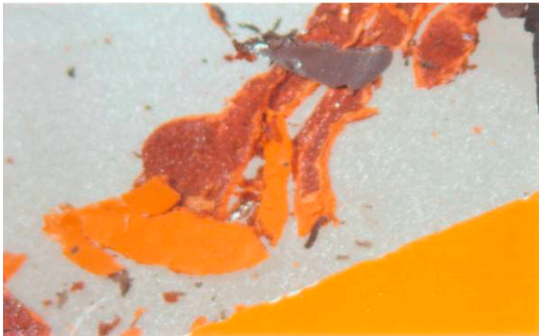
Fig. 4 Original Orange-Colored Finish and Primers Found on Interior Metal Trim of Wright Brothers National Memorial Visitor Center (Munsell Color Chip 2.5YR 6/16 Visible in Lower Right Corner of Photograph), (2000).
