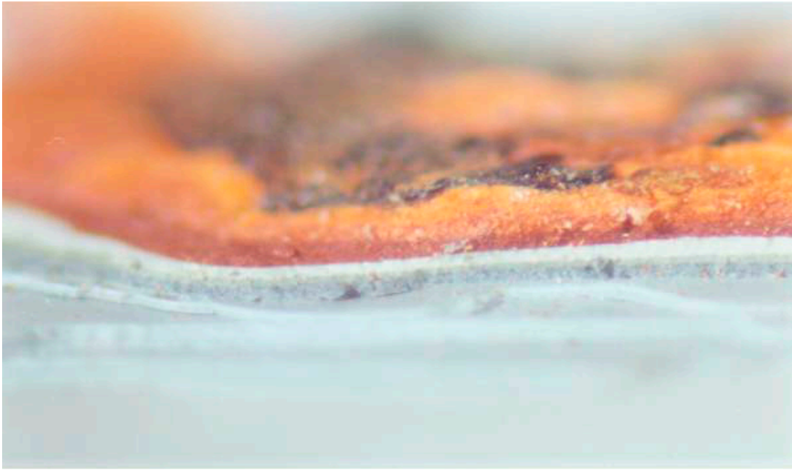
Fig. 3 Paint Sample WRBR-VC-P003 removed from Fence Post East of Wright Brothers National Memorial Visitor Center, Viewed at 30x. Note Original Orange Finish and Primer Coats. Later Red-Colored Finish is Believed to Date from Late 1960's or Early 1970's, (2000).
