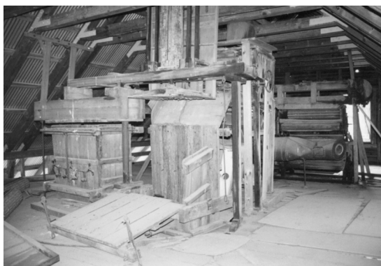
Figure 44 View east of dual-box, hydraulic press at second floor, with gin stand visible in background. (NPS-SERO-CRS, 2001)
