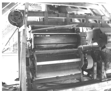
Figure 41 View of Continental gin stand on second floor. (NPS-SERO-CRS, 2001)
